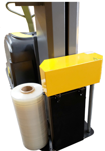
Pre-stretch carriage saves up to 40% on film costs
